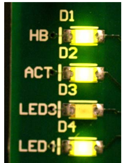
Fig.6: Distribution Board LED's
