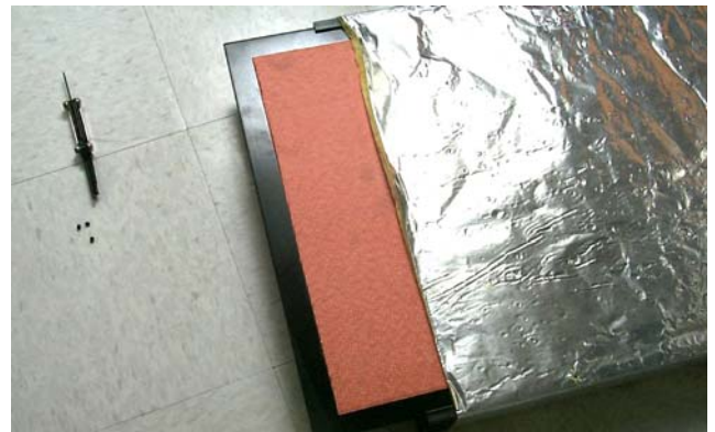
Fig. 13: The heater plate slides from the insulation.
